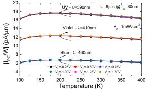
Fig. 8. Normalized absolute photocurrent,  $|I_{PG}/W|$  under UV, violet and blue illumination, as a function of the temperature for photodiode with Li=8 $\mu m$ .
