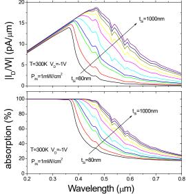
Fig. 12. Normalized absolute total current,  $|I_D/W|$  and absorption for different silicon film thickness (t<sub>si</sub>) as a function of wavelength ( $\lambda$ ) for photodiode with  $L_i=5\mu m$ .
