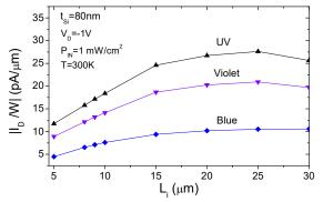
Fig. 10 Normalized absolute total current  $|I_D/W|$  under UV, violet and blue illumination, as a function of intrinsic length.
