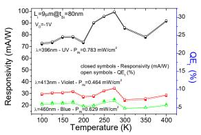
Fig. 6 Responsivity and total quantum efficiency under different light sources, as a function of the temperature for the studied photodiode.
