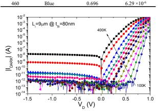
Fig. 3 Absolute dark current measured for temperatures between 100K and 400K, as a function of the applied voltage.
