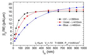
Fig. 14. Normalized absolute total current,  $|I_D/W|$  under UV, violet and blue illumination, as a function of silicon film thickness.
