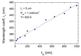
Fig. 13 Wavelength cutoff as a function of silicon film thickness.
