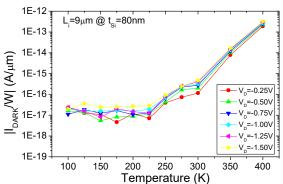
Fig 4 Normalized absolute dark current as a function of temperature measured at different applied voltages.
