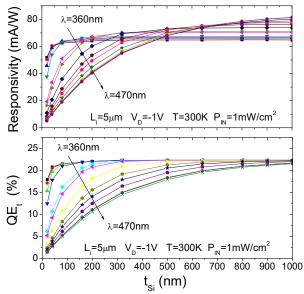
Fig.15 Responsivity and total quantum efficiency under UV, violet and blue illumination as a function of silicon film thickness.
