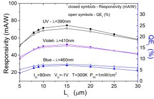
Fig. 11 Responsivity and total quantum efficiency under UV, violet and blue illumination as a function of intrinsic length region.
