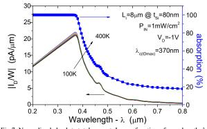
Fig.7 Normalized absolute total current,  $I_D$  as a function of wavelength,  $\lambda$  for the temperature range of 100K to 400K for photodiode with  $L_i\!\!=\!\!8\mu m.$
