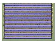
Fig. 2 Optical microscope top view of an interdigitated PIN SOI lateral photodiode used in this work [10].
