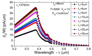
Fig. 9 Normalized absolute total current,  $|I_D/W|$  for photodiodes with different intrinsic length, as a function of the wavelength.
