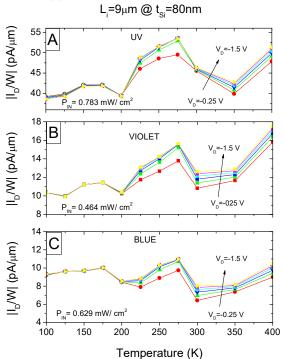
Fig 5 Normalized total current as a function of temperature measured at different applied voltages and three different light sources.
