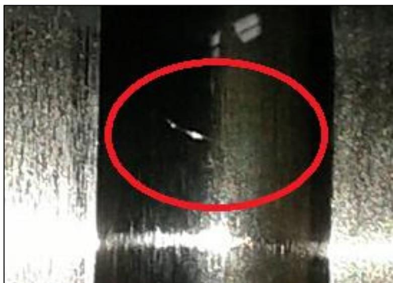
**Figura 102: Rolamento 01 – Pista Interna – Ranhura transversal ampliada**
