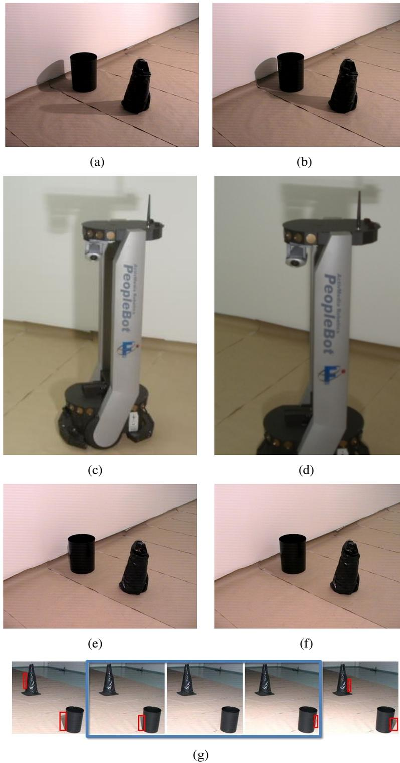
Figura 3.2: Imagens capturadas pelo *PeopleBot*<sup>TM</sup>. Representando as relações PQRS (a) NonOccludesDC(o,s), (b) NonOccludesEC(o,s), (c) PartiallyOccludesPO(o,s), (d) PartiallyOccludesTPP(o,s), (e) TotallyOccludesTPPI(o,s), (f) TotallyOccludesEQ(o,s) e (g) TotallyOccludesNTPPI(o,s).
